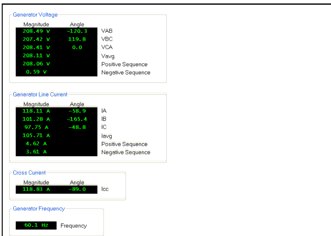
Figure 58. Generator Primary-Values Metering
