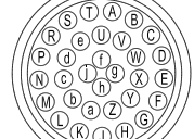
ME connector (32 pin) Glennair IPT 02 A 18-32 P F6 front view
