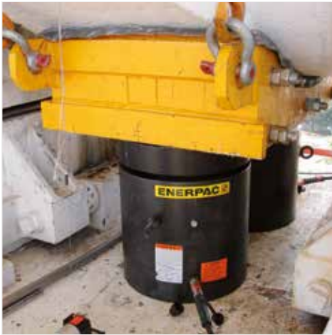
▲ Heavy lifting and foundation leveling. The lock nut provides mechanical load holding over a long period of time.
