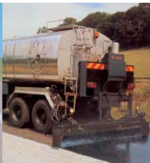
Cold-binding-agent spraying machines and vehicles with spraying ramps
