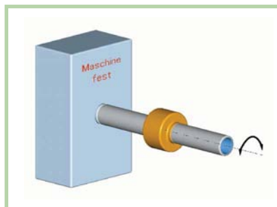
Slow rotary movement with type 11S (1 fixed point, 1 side flexible)
