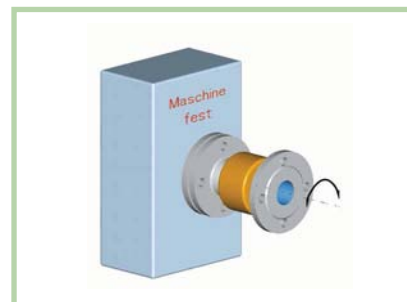
Slow rotary movement with type 11F (1 fixed point, 1 side flexible)
