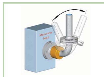
Swivel movement with type 12F (1 fixed point, 1 side flexible)
