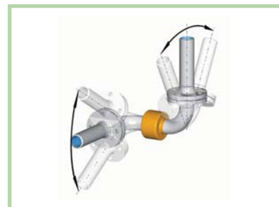
Swivel movement on both sides with type 13F in angled pipe piece
